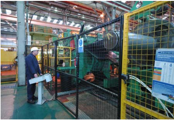
ABOVE: The line’s decoiler can be controlled independently via its own free-standing console.
